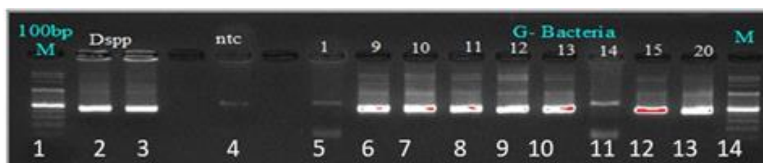
Fig.1. Agarose gel electrophoresis for PCR. Amplified 430 bp product. Lane 1,14 - 100bp DNA ladder, Lane 2,3, positive control, 4- negative control, Lane 5,6,7,8,9,10,11,12,13 –bacterial strain
